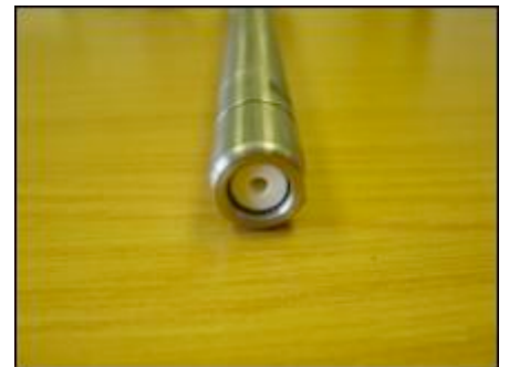
Figure 2: SpringSparge Sparger and sealing port arrangement
