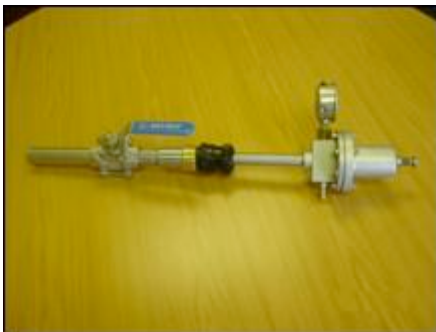
Figure 2: SpringSparge Sparger and sealing port arrangement
