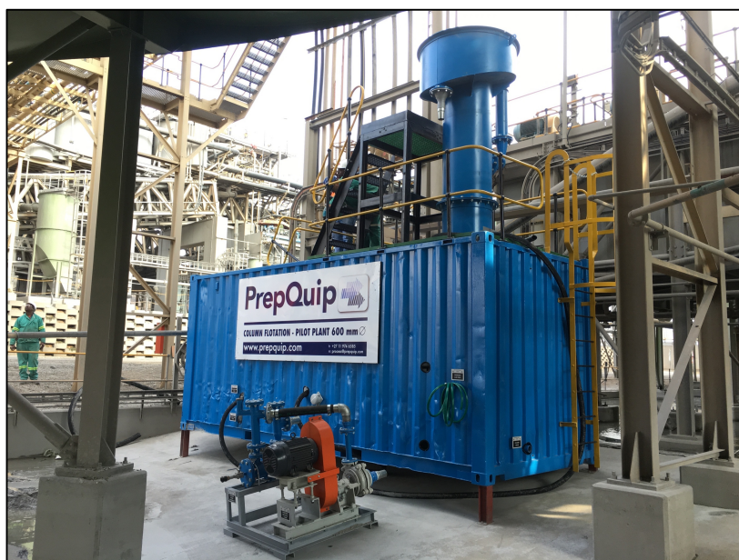
Figure 2: PrepQuip column flotation pilot plant (600 mm)
